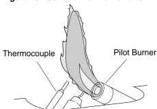
Figure 19 - Incorrect Pilot Flame Pattern
